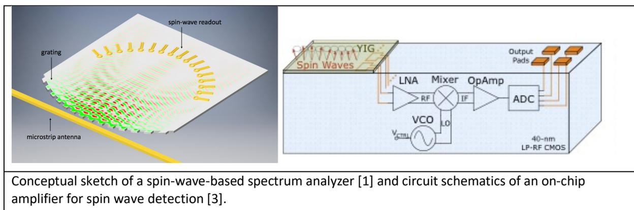
Conceptual sketch of a spin-wave-based spectrum analyzer [1] and circuit schematics of an on-chip amplifier for spin wave detection [3].
